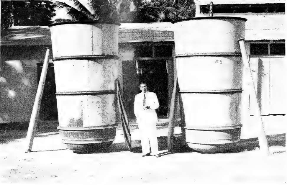
FIGURE 11.—Stills used in Haiti for the processing of lemon grass.
